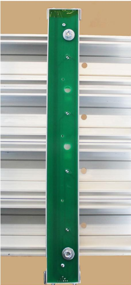
Slide the timer over the end of the track with the sensor bar beneath the track. Place the timer over the bolts installed in the previous step using the **timer's** track mounting holes (holes shown in picture on previous page). Then place a washer over each bolt and secure the timer with an additional nut on each bolt. **Finger tighten only. Do not over tighten.**
