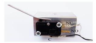
If you want the switch to be un-pressed before the race and pressed when the race starts, then the push-on terminal needs to be on the NO contact as indicated below.
