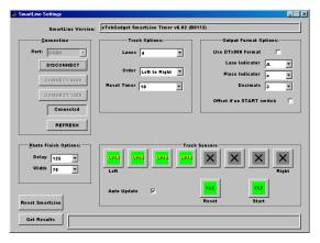
This is the display as it appears when there are 4 lanes and communication has been established successfully. Waving a hand under the sensors triggered the timer and the 'Get Results' button was pressed in order to see the result string from the timer.
