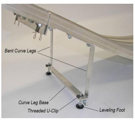
Install leveling mounts with leveling feet at the bottom end of the curve section as you did with the straight section. Attach these at the bottom end of your curve section as in the previous section.
