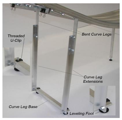
Using four ¼-20 X ½" hex bolts and nuts, bolt the curve leg extensions onto the curve legs as shown. Now bolt the curve leg base to the bottom of the extensions using two ¼-20 X ½" hex bolts and nuts. Slide two threaded U-Clips onto the Curve Base so that they snap into the large holes at each end. Thread a leveling foot into each U-Clip.
